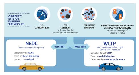
An overview of the differences between the NEDC and its replacement, the WLTP.
