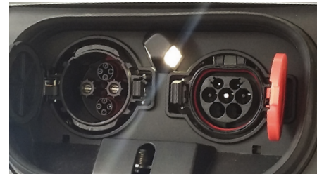
Nissan Leaf charging sockets. Nissan and Mitsubishi EVs use separate sockets for AC and DC charging. The AC socket is on the left and the CHAdeMO DC socket is on the right. Currently, public DC charging stations in Australia have leads for both CCS2 and CHAdeMO charging.
