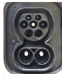
CCS2 charging socket. CCS2 is the socket type used on most of the new crop of EVs in Australia, and includes AC and DC charging in the one socket (AC at the top and DC at the bottom).
