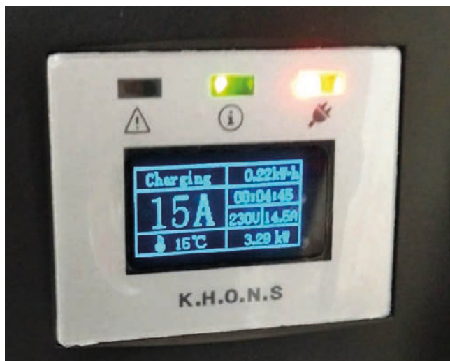
Portable EVSEs usually have basic features. Some have no display except for LEDs, while others have small screens that supply charging and operating information.
