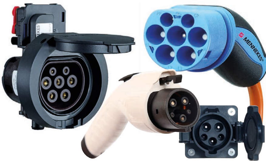
The Type 2 (Mennekes) socket is now the standard for EVs in Australia, although some older EVs—like the beige one pictured here—will come with a Type 1 (J1772) socket (pictured bottom right). If your EV has the latter, then you will need an EVSE with a Type 1 plug, or suitable adaptors.
